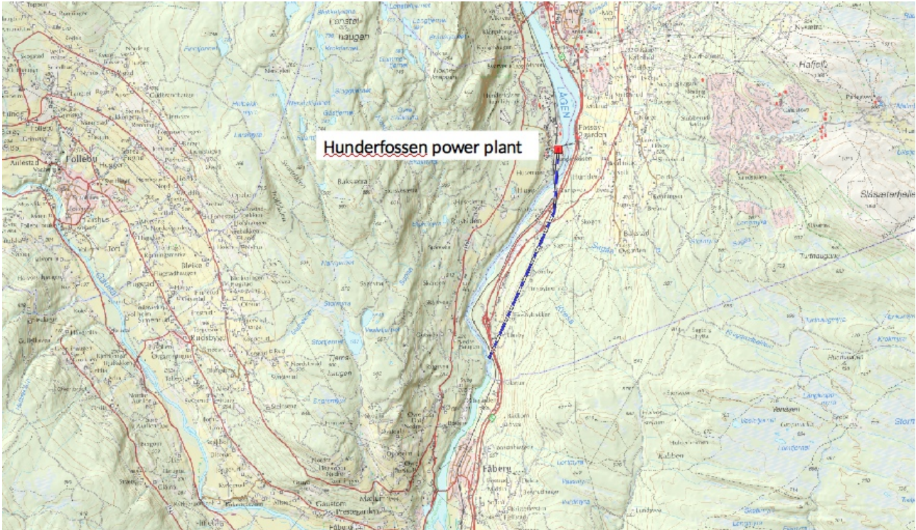
Figure 2. Hunderfossen power plant (red square) on the main stem of Gudbrandsdalslågen river. Dashed line is the power production tunnel, indicating the intake and outflow. Map reproduced with permission from the owners.
